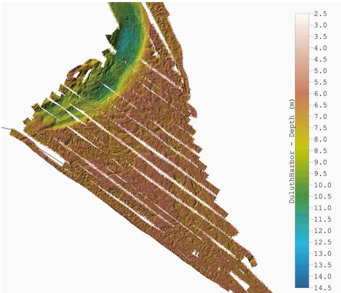
Figure 4: Multibeam bathymetry data for the East Gate Basin.
