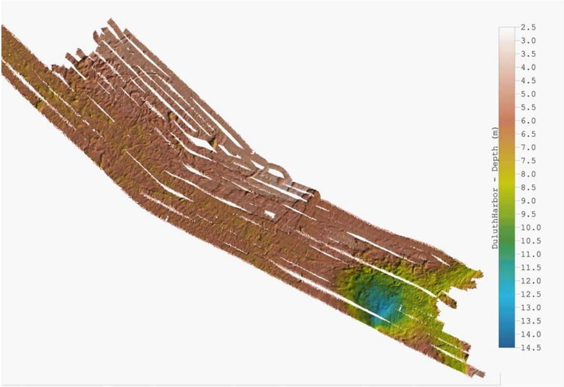
Figure 6: Multibeam bathymetry data for the Superior Harbor Basin.
