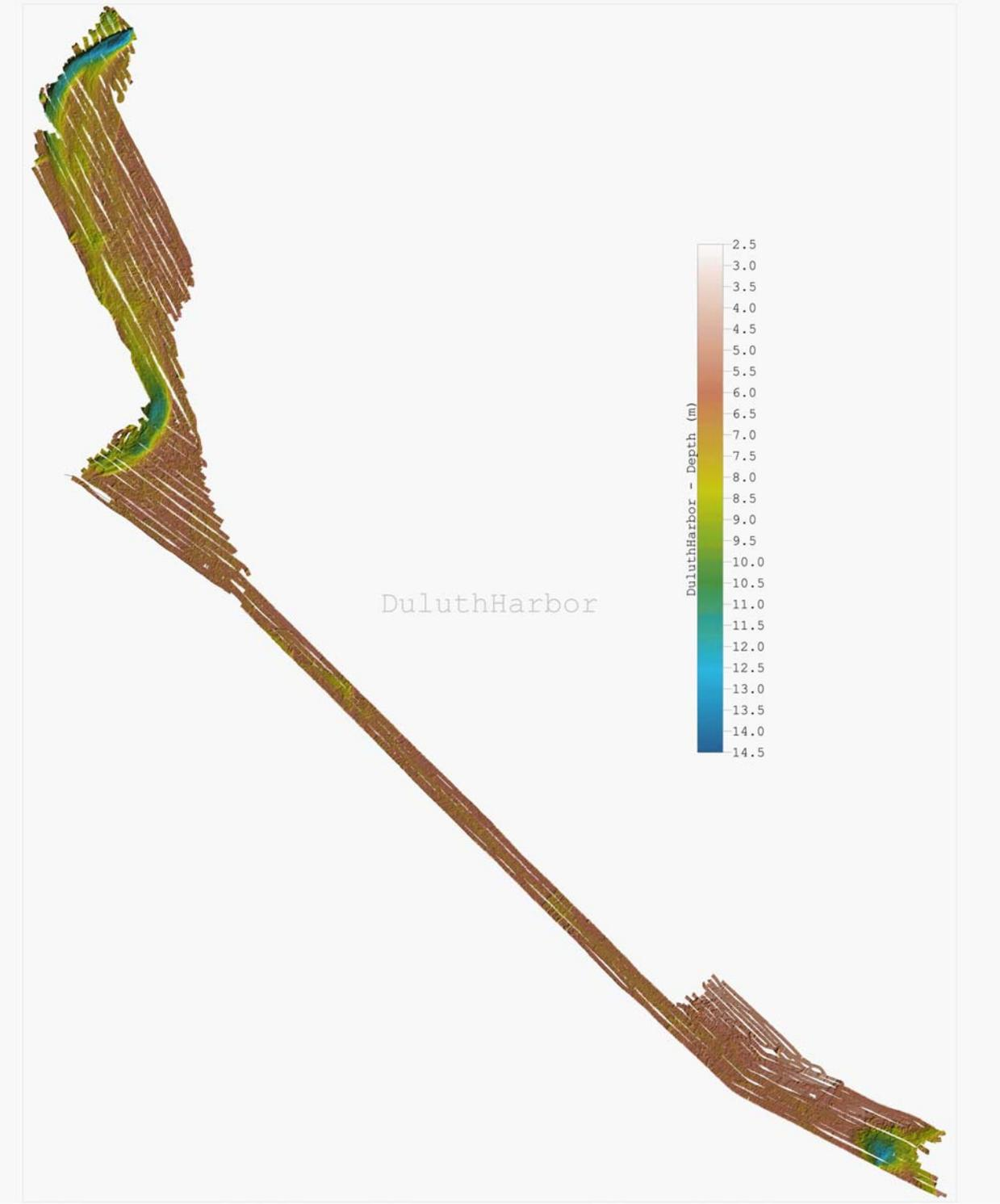
Figure 2: Multibeam bathymetry data for the Duluth-Superior Harbor.
