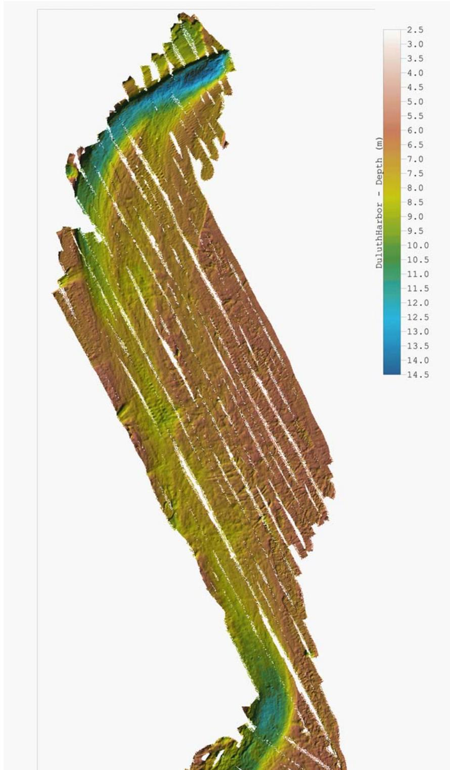
Figure 3: Multibeam bathymetry data for the Duluth Harbor Basin.
