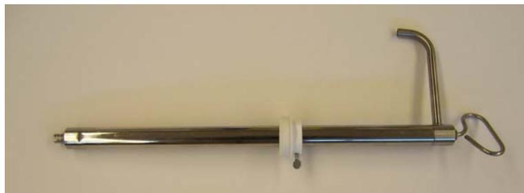
**Figure 5: Stainless-steel drum pump.**
