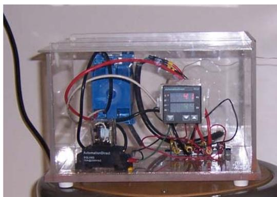
**Figure 2: Temperature controller unit.**
