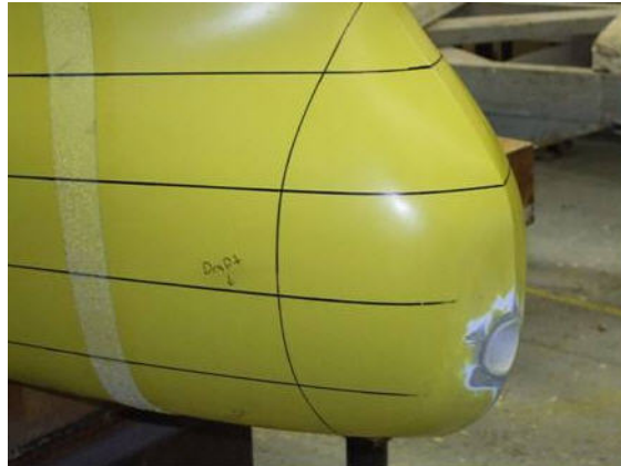
Figure 2.5: Location of Forward Ballast Trunk Inlet
