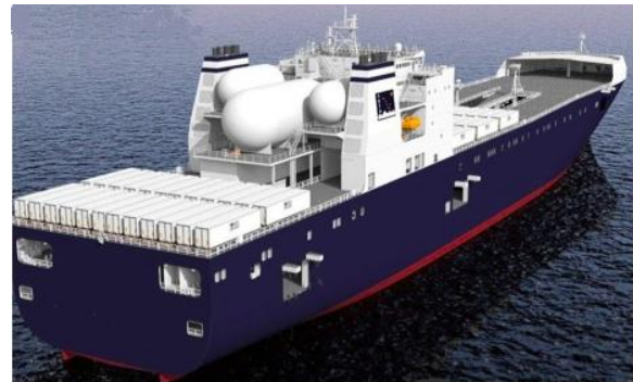
Figure 8. TOTE's dual-fuel LNG containership retrofit for Alaska Service. Image courtesy of TOTE.
