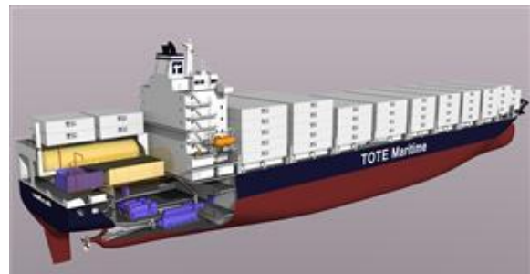
Figure 9. TOTE Shipholdings new LNG containership for Puerto Rico service. Image courtesy of TOTE.
