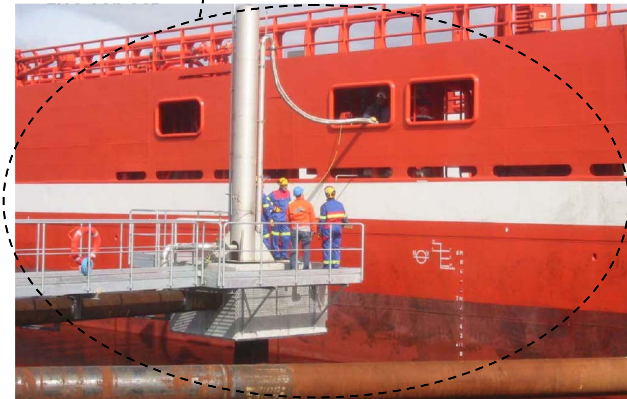
Figure A2. Close up of quayside LNG bunkering
