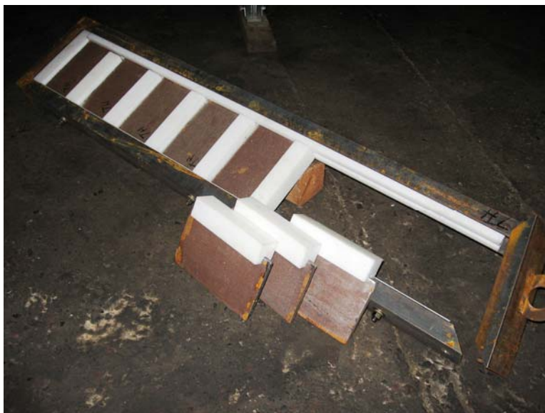
Figure 2. Photograph of metal tray frame and sheet steel coupons (separated by white HDPE spacers) before being installed in the Duluth-Superior Harbor during October 2006. [Photograph courtesy of AMI Consulting Engineers]
