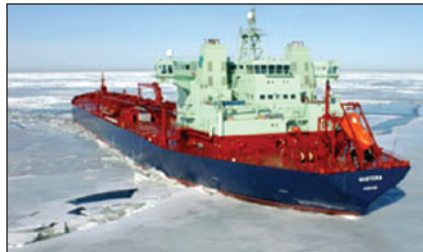
The "double-acting" icebreaker Mastera breaks ice while going backward.
