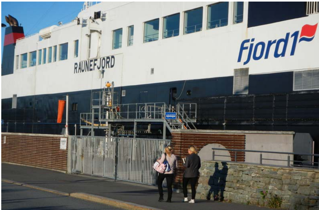
Figure 11 LNG Refueling Location Adjacent to Walkway
