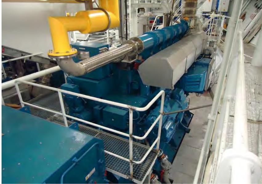
Wärtsilä dual fuel 6L34DF generator set onboard the PSV *Viking Princess* with double-walled gas supply line in yellow
