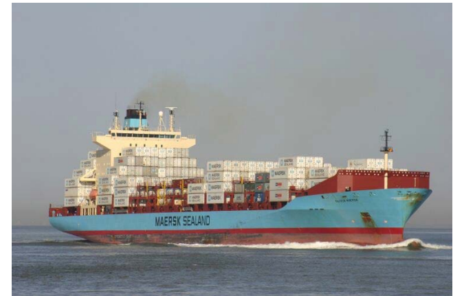
The Olivia Maersk ( L = 238 m) was equipped with an air lubrication system based on “WAIP” technology developed in Japan.
