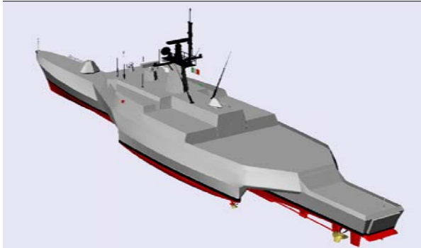
2,200 t Trimaran Offshore Patrol Vessel/Frigate
